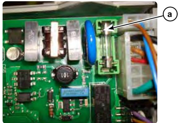
**Figure 116** Thermostat-relay circuit fuse location
