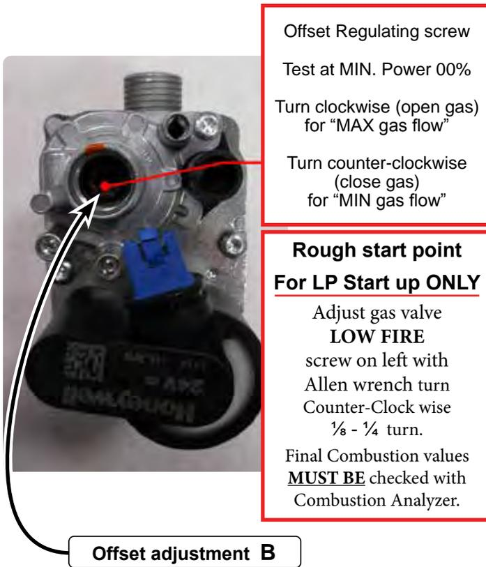
**CAUTION** Adjust in steps of no more than 1/8 of a turn and wait 1 minute after each adjustment to allow the setting to stabilise. Turning the screw too far will cause the adjustment to reverse behavior.
