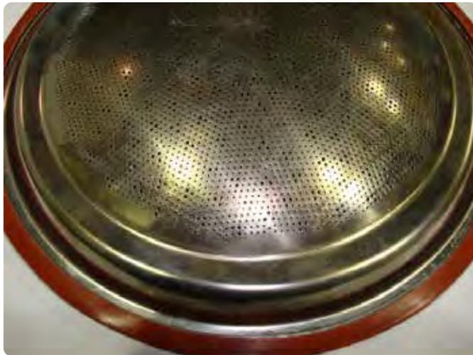
7. **Inspect the burner exterior. It must be in good condition, with no visible damage.**
