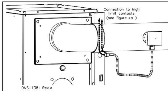
Figure 7: BVSO Wiring (OPTIONAL)
