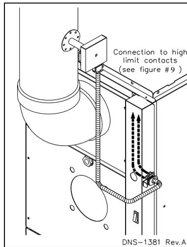
**Figure 6: BVSO mounting installation: Upflow with horizontal exhaust (OPTIONAL)**
