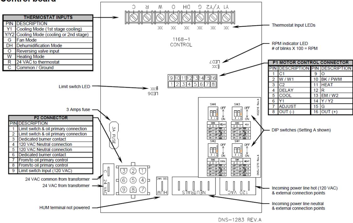
Motor control wires
