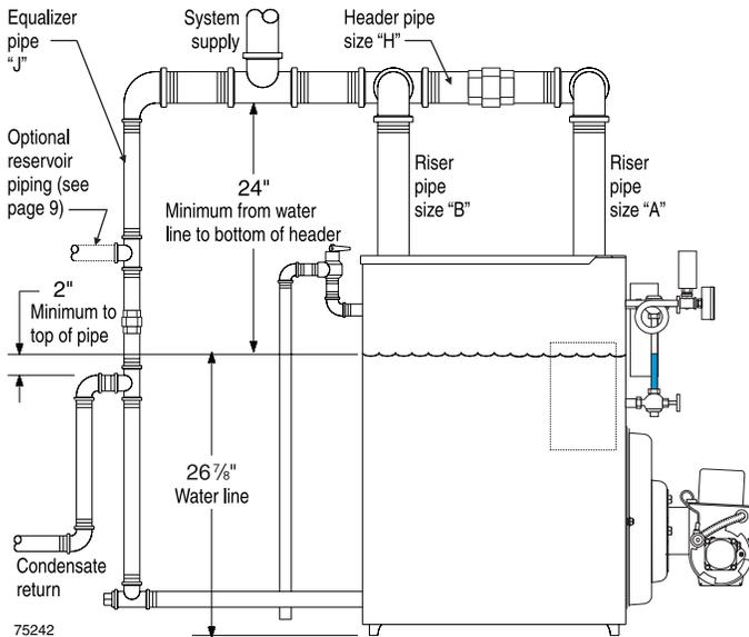
**Figure 7** Recommended piping, OSB-6, piping for parallel-flow systems only
