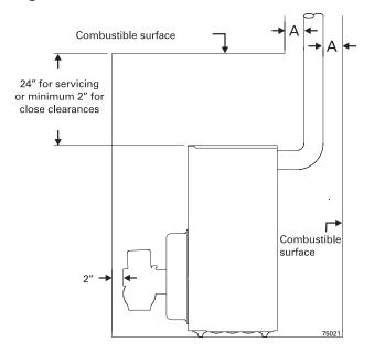
Figure 14 Protection required for close clearance
