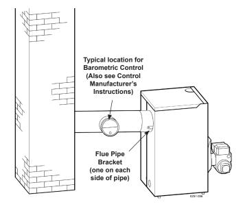
Figure 2b Top outlet breeching connection (only with optional "Top Vent Service Kit").
