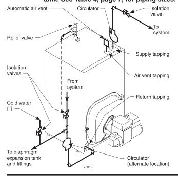
Figure 4 Closed-type expansion tank: Piping to single-zone system using closed-type expansion tank. See Table 4, page 7, for piping sizes.
