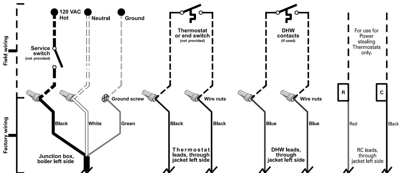
**NOTICE** Boiler circulator is shipped loose, with wiring harness connected and wired to boiler. After circulator is piped, connect wires to circulator and secure harness conduit connector to circulator junction box.
