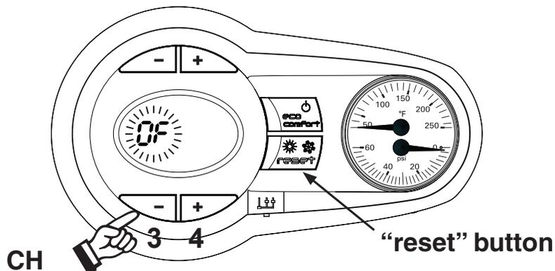
3. Switch to OF (Offset mode) by pressing the CH + or – buttons (Items 3 and 4 - above). The display shows “OF” flashing
