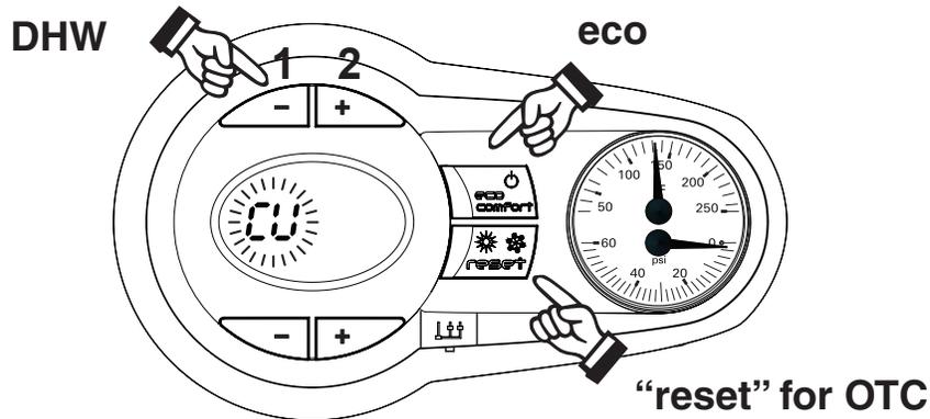
1. To enter the OTC - reset mode, press “reset” button for 5 seconds, takes you to Curve menu.
