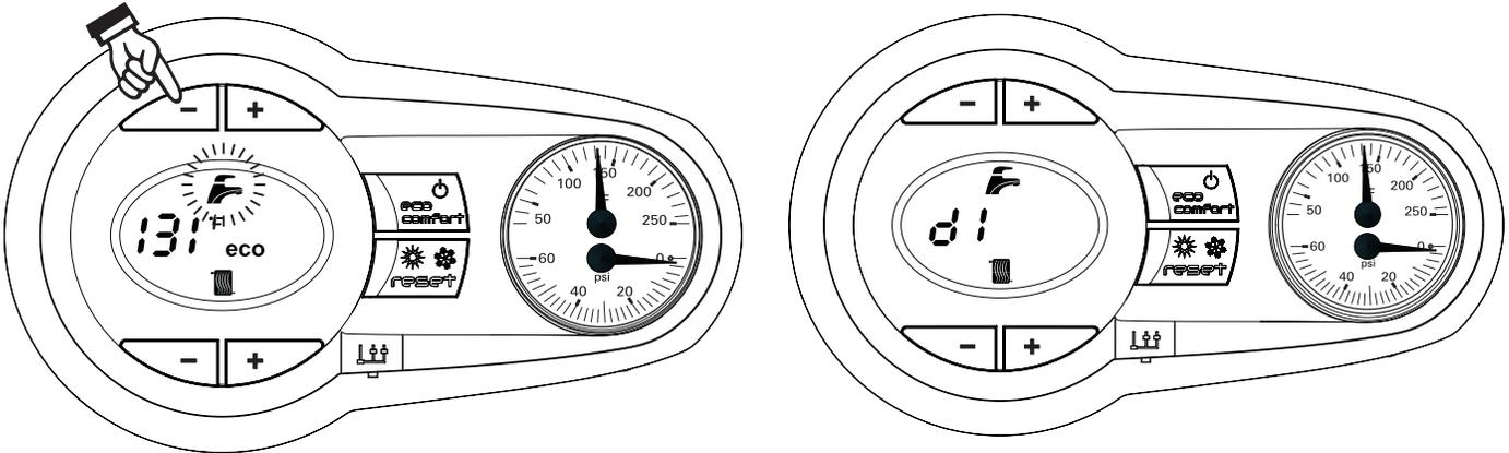
To set the Domestic hot water temperature, use the DHW buttons, “-” to reduce water setpoint “+” to increase water setpoint. It can be set from a minimum of 104° F to a maximum of 131° F.
