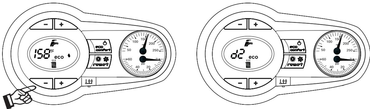
To set the system Heating temperature, use the CH buttons, “-” to reduce water setpoint “+” to increase water setpoint. It can be set from a minimum of 68° F to a maximum of 190° F.
