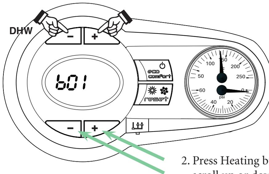
2. Press Heating buttons + & - to scroll up or down the parameter numbers
