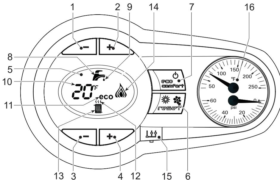
1. When the external outdoor sensor is attached to the boiler, the system can work in Outside Temperature Compensation mode. In OTC mode the temperature of the heating system is controlled according to the external climate conditions, this will insure a high degree of comfort and Energy saving all year round.
