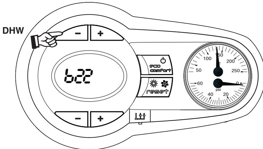
Exiting the “User interface setting” menu. Press the “DHW +” and “DHW -” buttons together for 10 seconds; or switch the power to the unit off and then on again; or wait for automatic exiting which occurs after two (2) minutes
