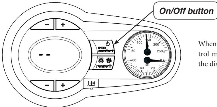
When the boiler is turned off with “eco”/power button, the control module is still powered, heating operation is disabled and the display is off, however the frost protection will still be active.
