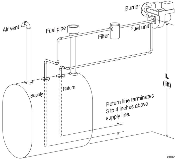
**Table 4** Two-line fuel system maximum lengths for 3/8" and 1/2" OD copper tubing distribution. Use only for burners equipped with Suntec fuel units. See fuel unit data sheet for any other fuel unit.
