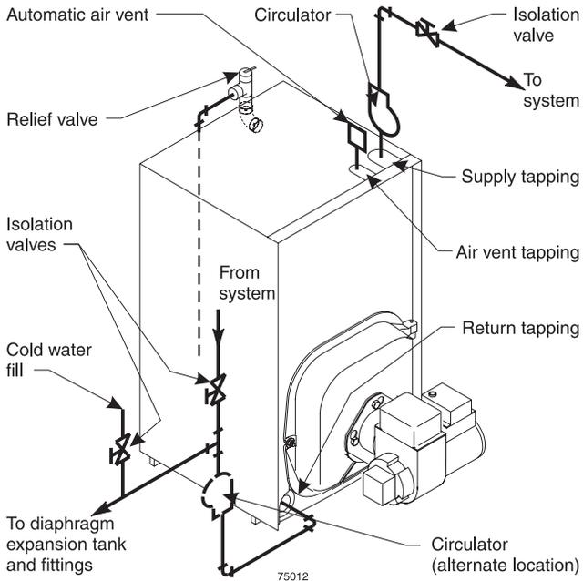
**WARNING** Use Figure 3 or Figure 4 only for systems designed for return water at least 130 °F. For systems with low return water temperature possible, such as converted gravity systems and radiant heating systems, install by-pass piping (see page 9) to protect boiler against condensation. Failure to prevent low return water temperature to the boiler could cause corrosion of the boiler sections or burners, resulting in severe personal injury, death or substantial property damage.
