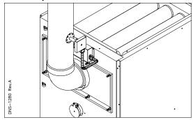
Figure 2 Blocked Vent Shutt-Off device wiring Upflow with Horizontal exhaust
