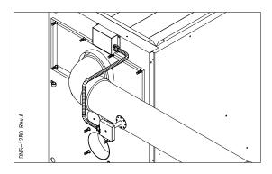
Figure 3 Blocked Vent Shut-Off device wiring Horizontal left/right with Vertical exhaust
