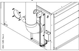
Figure 4 Blocked Vent Shut-Off device wiring Horizontal left/right with horizontal exhaust
