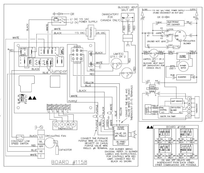
STANDARD HEAT / COOL WIRING DIAGRAM WITH ELECTRONIC FAN TIMER WHEN HEATING & COOLING SPEED ARE THE SAME
