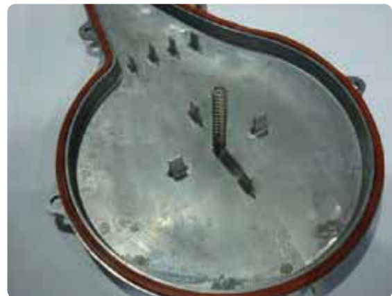
Figure 140 Heat exchanger cover plate removed
