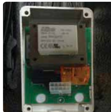
Figure 63 Thermostat-Relay box terminals Combi and Central Heating boilers
