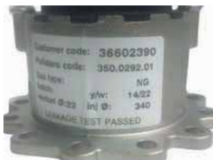
Figure 9 Natural gas venturi label information
