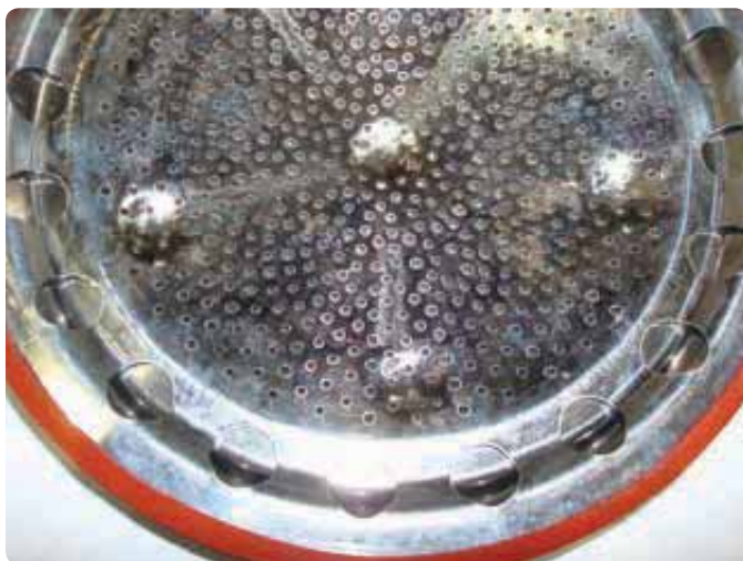
Figure 142 Inspecting interior and cleaning the burner
