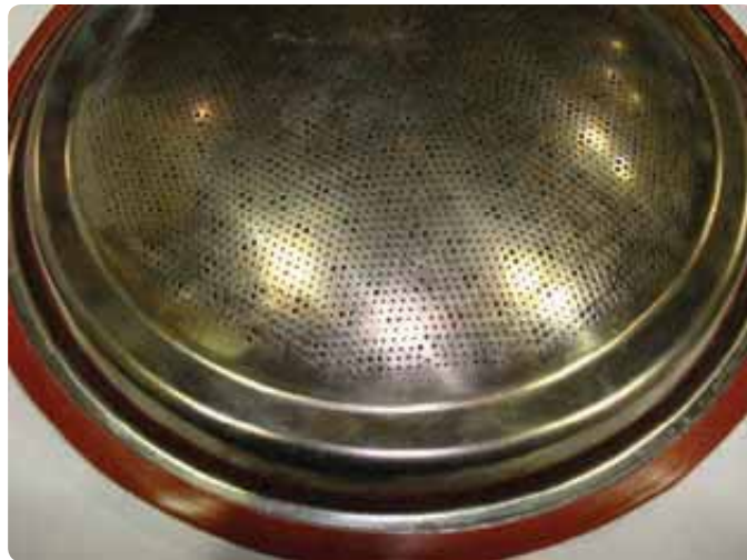
Figure 143 Inspecting exterior and cleaning the burner
