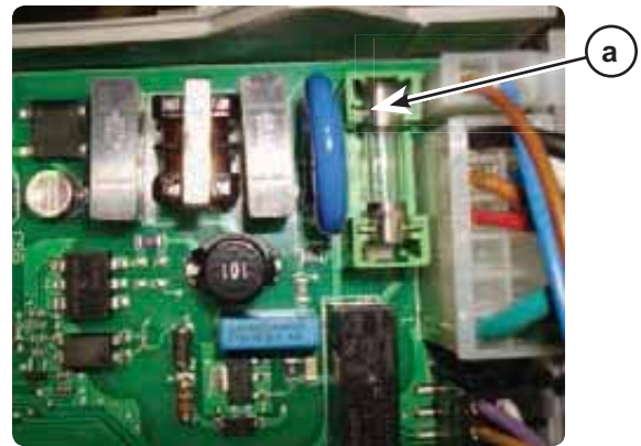
Figure 111 Thermostat-relay circuit fuse location
