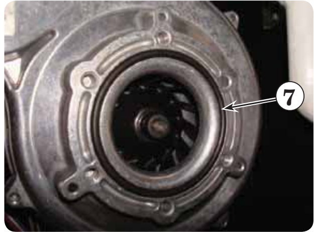
Figure 15 Insure "O" ring is in place
