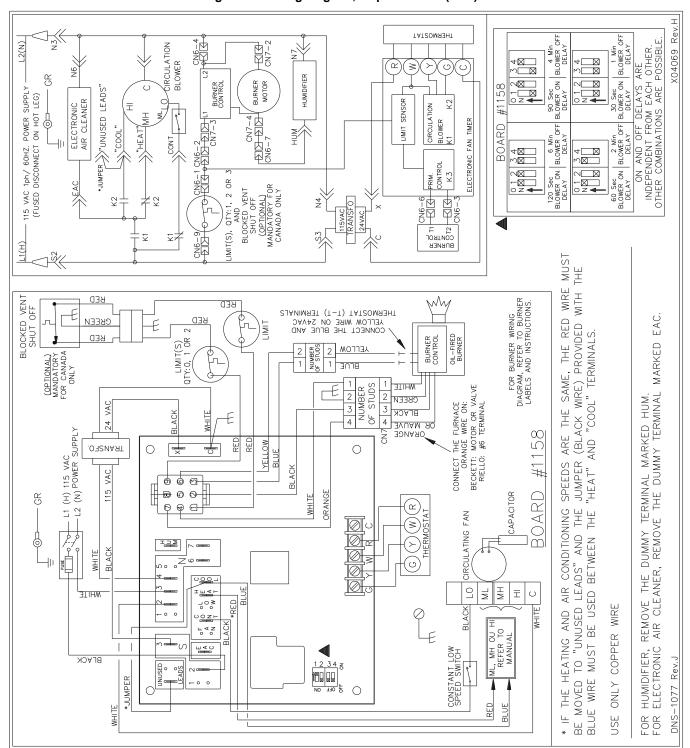
Figure 12: Wiring diagram, 4-speed motor (PSC)
