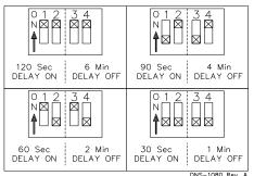
**SUPPLY AIR ADJUSTMENTS** 1.12. (ECM VARIABLE SPEED MOTORS)
