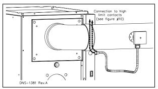
Figure 10: BVSO Wiring (OPTIONAL)
