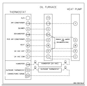
Note: On units with 2 stage cooling or heat pump, terminal Y1 must be used. When Y1 on the electronic control receives a 24 VAC signal, the air flow is reduced by 20%. Do not use terminal Y1 with a single stage cooling or heat pump.
