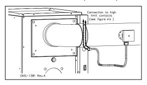
Figure 7: BVSO Wiring (OPTIONAL)
