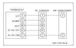
Figure 3: Thermostat Wiring- Heating & Air Conditioning - With ECM Variable Speed Motor
