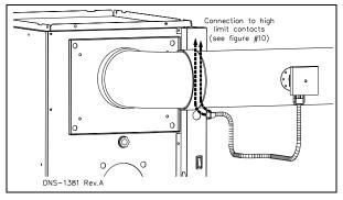
Figure 7: BVSO Wiring (OPTIONAL)
