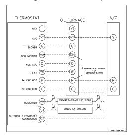
Figure 4: Thermostat Wiring-Heating & Air Conditioning / Heat Pump - With ECM Variable Speed Motor
