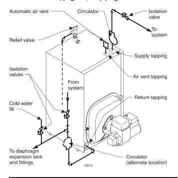
Figure 8 Closed-type expansion tank: Piping to singlezone system using closed-type expansion tank. See Table 4, page 10, for piping sizes.
