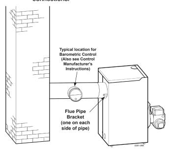
Figure 4 Top outlet breeching connections (only with optional "Top Vent Service Kit").
