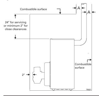
Figure 19 Protection required for close clearance
