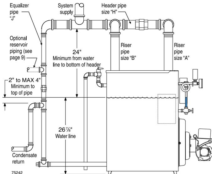
**Figure 9** Recommended piping, OSB-6, piping for parallel-flow systems only
