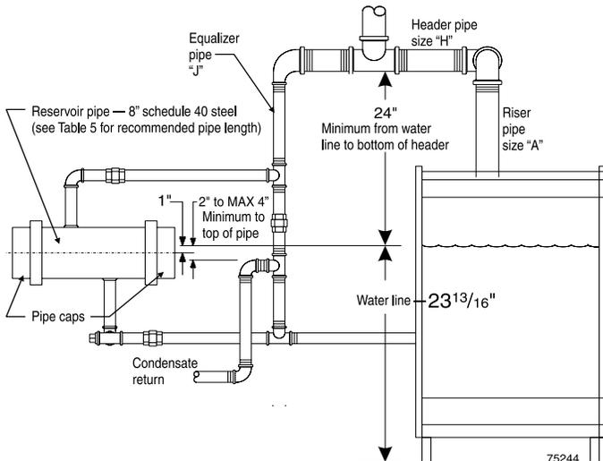
**Figure 11 Recommended piping for parallel-flow systems with optional reservoir pipe**
