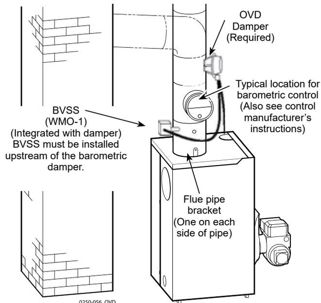
**Figure 3** Back outlet breeching connection for OSB-3 through 6 with OVD Damper.
