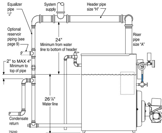
**Figure 7** Recommended piping, OSB-3, -4 and -5, piping for parallel-flow systems only
