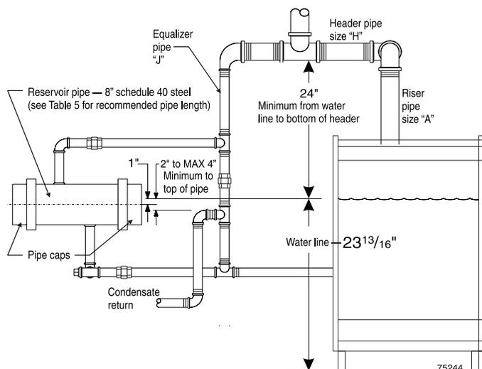
**Figure 9 Recommended piping for parallel-flow systems with optional reservoir pipe**
