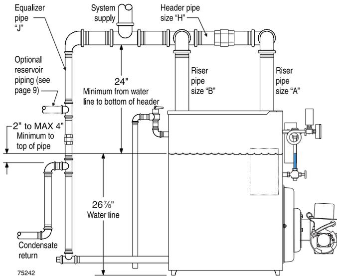
**Figure 7 Recommended piping, OSB-6, piping for parallel-flow systems only**
