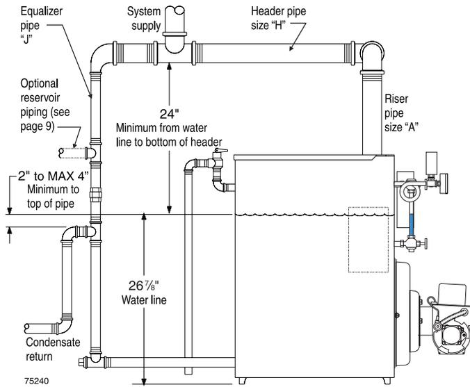
**Figure 5 Recommended piping, OSB-3, -4 and -5, piping for parallel-flow systems only**
