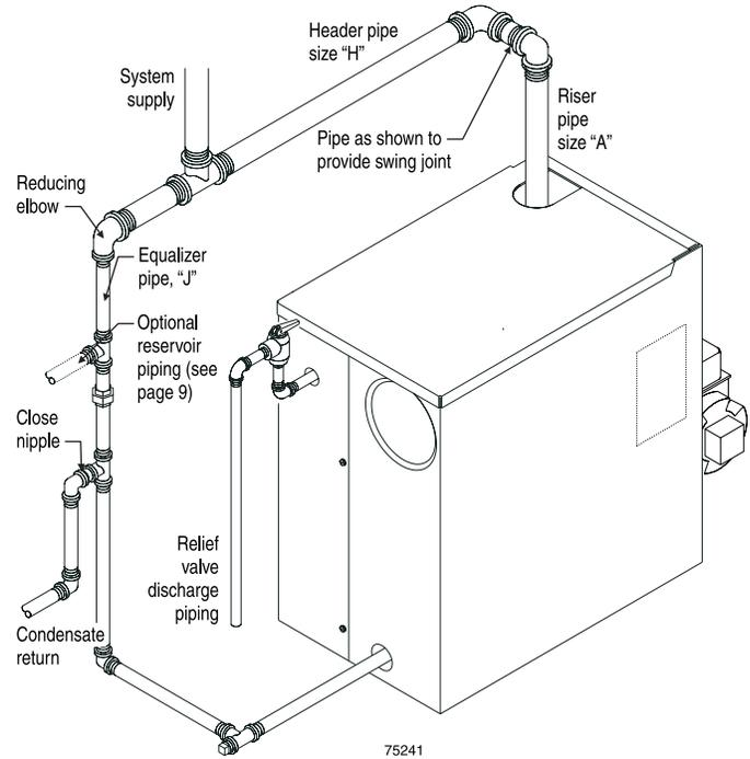
**Figure 6 Recommended piping, OSB-6, piping for parallel-flow systems only**
