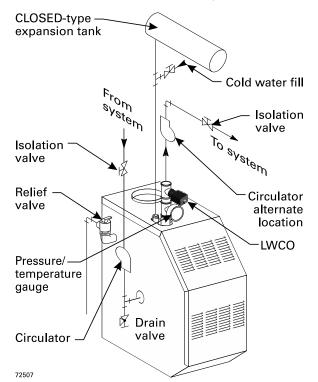
▲WARNING Use Figure 5 or Figure 6 only for systems designed for return water at least 130 °F. For systems with low return water temperature possible, such as converted gravity systems and radiant heating systems, install bypass piping (see **page 12**) to protect boiler against condensation. Failure to prevent low return water temperature to the boiler could cause corrosion of the boiler sections or burners, resulting in severe personal injury, death or substantial property damage.
