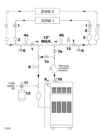
Figure 13 Primary/secondary piping Zoning with zone valves
