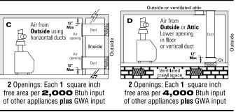
**EXCEPTION: NO** combustion air openings are needed when the boiler (and other appliances) are installed in a space with a volume **NO LESS** than 50 cubic feet per 1,000 Btuh of all installed appliances. Sum the total input of all appliances in MBH (1,000's of Btuh) and multiply this number times 50. *Building must not be of Tight construction* (see below).
