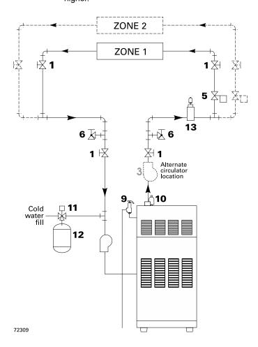
10Automatic air vent (with diaphragm-type expansion tank), or connect to tank fitting (closed-type expansion tank). DO NOT use an automatic air vent when using closed-type expansion tank. It would allow air to leave the system, causing waterlogging of the expansion tank.
