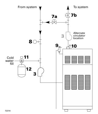
System-bypass piping as shown in Figure 16 can be used with either zone valve or circulator zoning. When used with circulator zoning however, the boiler circulator (item 3), must be piped as shown. It cannot be used as one of the zoning circulators.
