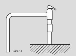
▲WARNING Plugging T&P relief valve or discharge piping can cause excessive pressure in the water heater, resulting in severe personal injury, death or substantial property damage.
