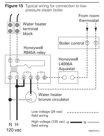
Install the Honeywell L4006A aquastat in the boiler, below the water line. Set for a temperature of 180 to 190°F to control boiler temperature when there is no call for steam heating.
