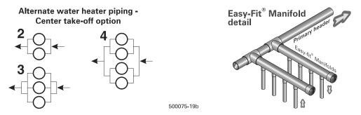
Figure 14 Multiple water heaters and dedicated multiple boilers — boiler water piping
